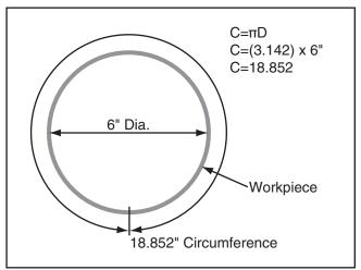
Figure 21. Calculating circumference example.
